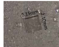
Figure 3: HPHT 2a (pure) diamond, <5ppm nitrogen present. The PL of this diamond is shown in Figure 5
