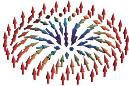
Figure 1: Model of a Neel-type Skyrmion, which is characterized by the spins rotating in radial planes from the core to the periphery. 4
