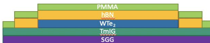
Figure 20 Side view of first spin coated stack
