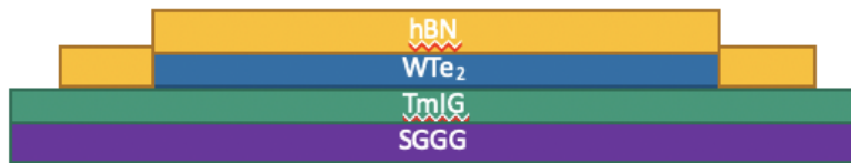
Figure 8 Side view of WTe_2/TmIG stack
